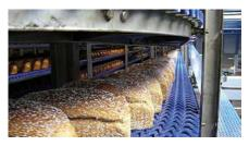
The belt surface of the JP link is not completely closed. Through the open area of the belt, fluids can fall to the ground, which enables the JP Link system to be used in wet environments. On a straight section the open area is 36% of the surface. The belt material is FDA approved.
