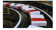
The JP Link system easily replaces several conveyors and expensive curves. In some cases the total belt length can be considerably reduced because only an upper part is needed.
