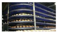
Thanks to the small inner radius of max. 1.3 times the belt width, the JP Link system can be installed in a confined space and used in almost every floor plan. JP Link ensures that products will leave your production line in a uniform manner. Even after several curves, your products will be ready for the following (automated) process.
