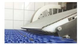
THE CLEATRAC TRANSFER IS DESIGNED TO CREATE A SMOOTH TAKE-OVER OF SMALL (FOOD) PRODUCTS, DUE TO THE FACT THAT THIS CONVEYOR HAS KNIFE EDGES ON BOTH SIDES. THIS CONVEYOR CAN BE USED FOR THE TRANSFER OF SMALL FOOD OR **NON-FOOD PRODUCTS.**
